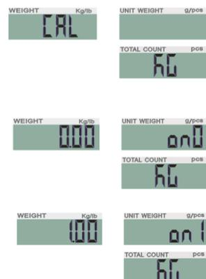
If you need to change the value, do as the following: Press key **G N/SET** to enter the value setting. Press key **◀/MR** or **TARE/▶** to move leftwards or rightwards. Press key **M-/HI** or **PRINT/LO** to modify the value (or via numeric keys). Press key
