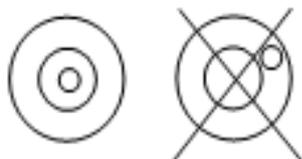
Note: The scale should be leveled each time its location is changed.
