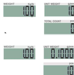
The unit weight is calculated, with Symbol “▼” pointing at “ACAL”.
