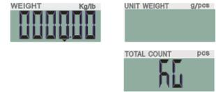
Preset-tare value setting: Press key **◀/MR** or **TARE/▶** to shift and key **M-/HI** or **PRINT/LO** to modify the value (or via numeric keys).
