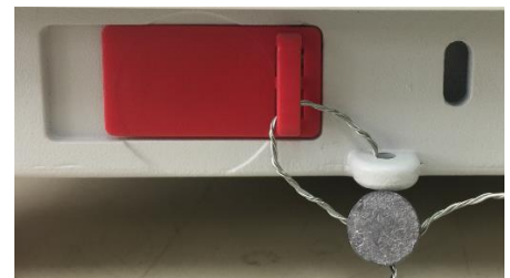
Locked with Wire Seal
