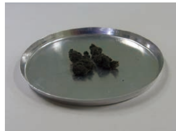
(Before measurement) The consistency was lumpy, so it was broken up using the tip of a spatula.
