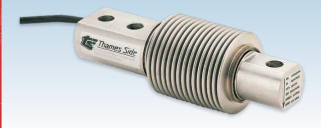
This fully welded stainless steel bending beam load cell is hermetically sealed to IP68 / IP69K and can be used in the harshest industrial environments. It is suitable for weighing platforms, bag fillers, belt weighers and tank weighing in the Food Processing, Chemical, Pharmaceutical and general Bulk Handling industries.
