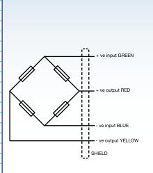
Electrical Connections /ia 4 wire, 6mm diameter, screened PVC cable.
