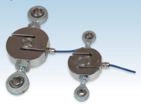
A range of Stainless steel "S" beam load cells for commercial weighing to OIML R60 3000 divisions. Welded construction ensures total environmental sealing coupled with excellent long term stability. A high temperature variant for operation in environments up to 150 °C is also available.
