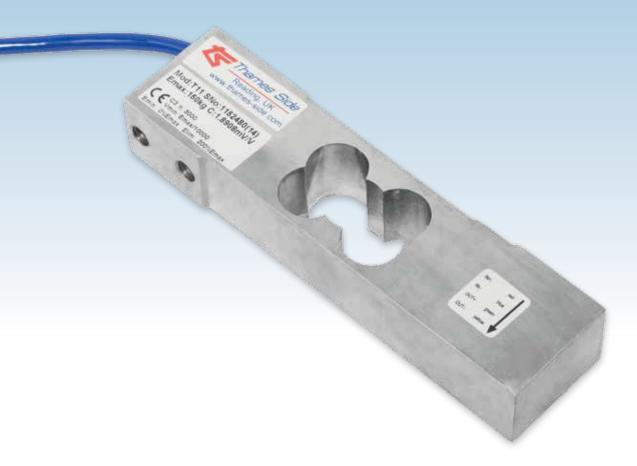
This double bending beam single point load cell is manufactured from high quality alloy steel and nickel plated. Its design allows for high accuracy weigh measurement with off-centre loads and it's potted and sealed to IP66.
