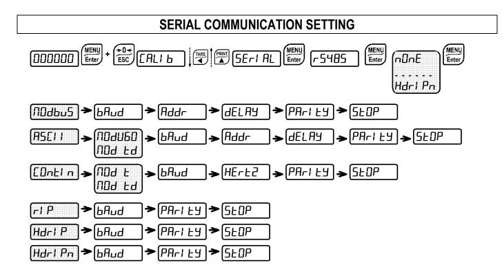
According to the chosen protocol only the necessary settings will be displayed in sequence (see diagram here above).
