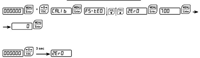
This menu may also be accessed directly from the weight display, holding down the key for 3 seconds.
