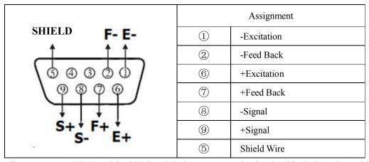
Short connect PIN 1 and 2, PIN 6 and 7 when connected a load cell with 4 wire cable;
