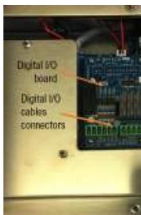
5 - Digital I/O PCB installed
