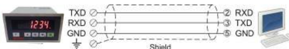
Figure 3.3 - RS 232C serial interface connections
