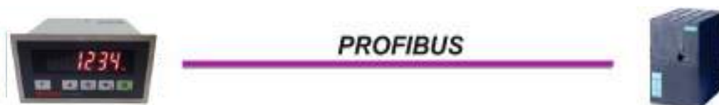
Figure 3.5 - FT-10 FILL PB serial interface connections
