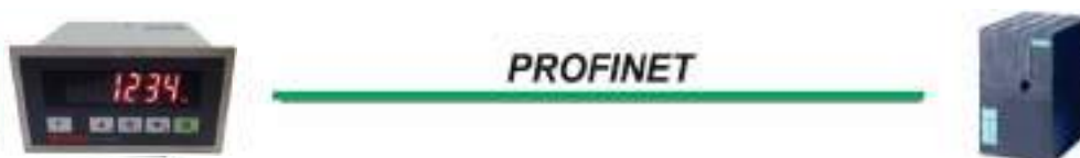
Figure 3.6 - FT-10 FILL PN serial interface connections
